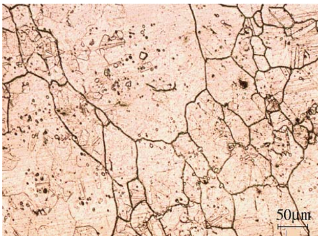
Fig. 7 Microstructure of the sample deformed at temperature of 1050 °C and strain rate of 0.5 s -1
